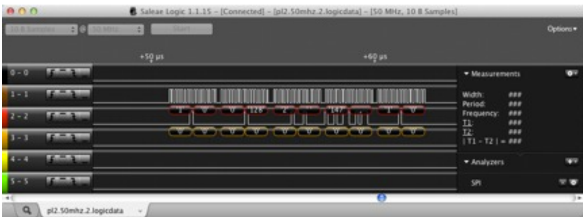
Figure 8: PL2 pin with SPI analyzer
