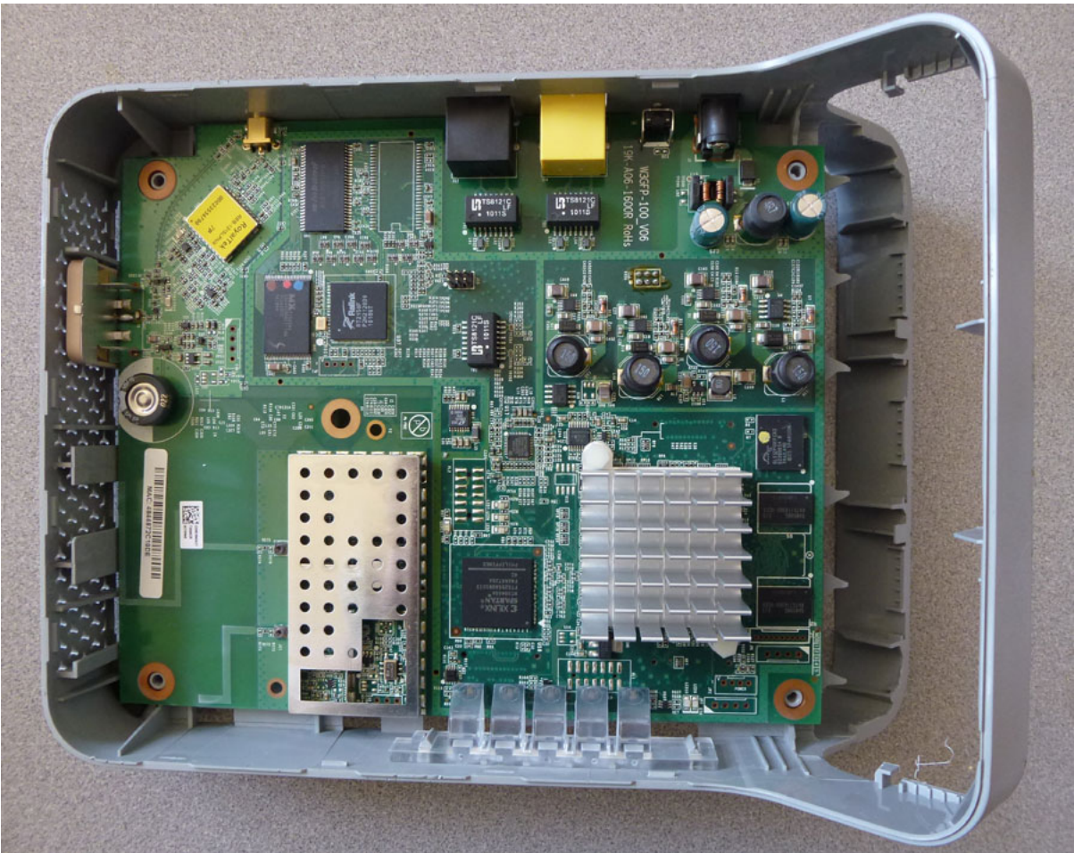
Removing four more screws, and popping more plastic tabs, enabled removal of the other side panel:
