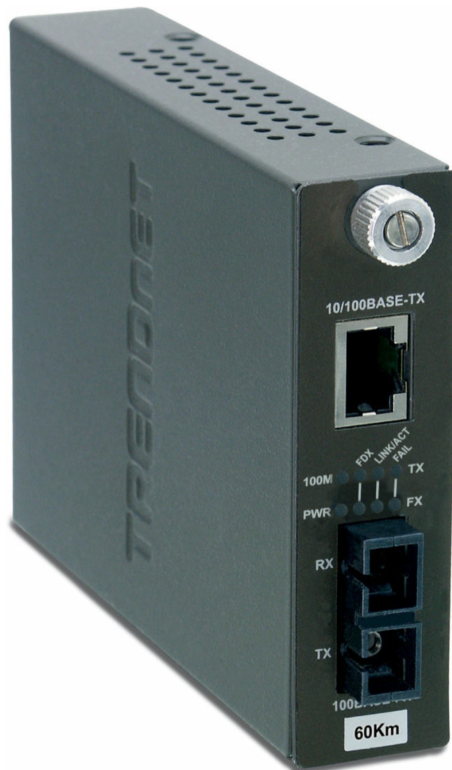
Figure 3-9 Typical copper-to-fiber Ethernet media converter (photo courtesy of TRENDnet)
