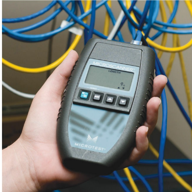
Figure 5-47 A typical medium-priced TDR called a MicroScanner
