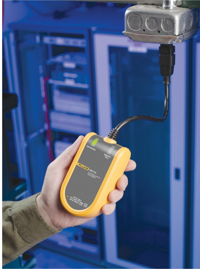
Figure 5-67 An excellent voltage event recorder (photo courtesy of Fluke Networks)
