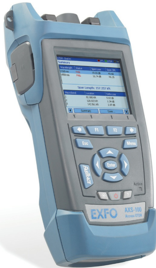
Figure 21-2 An EXFO AXS-100 OTDR (photo courtesy of EXFO)
