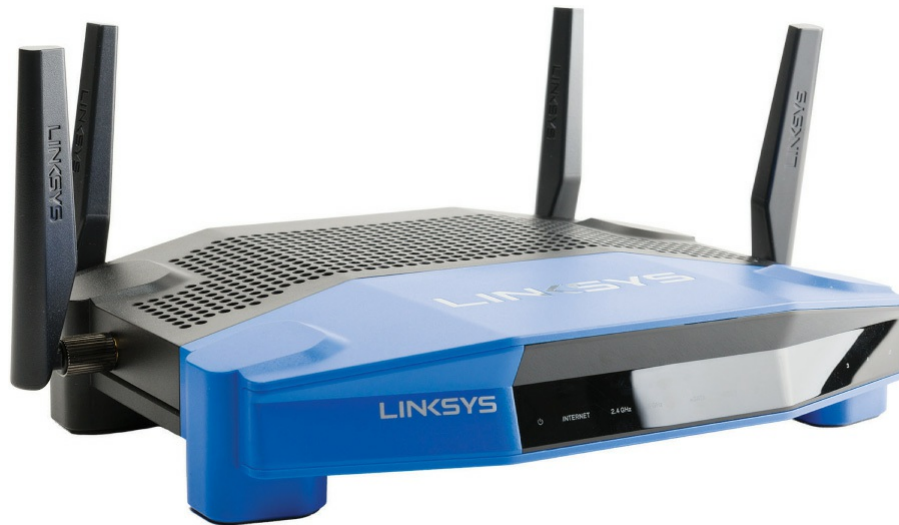
Figure 14-3 Linksys device that acts as wireless access point, switch, and DSL router
