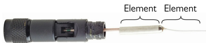
Figure 14-21 Typical WAP dipole antenna—where are the two elements?
