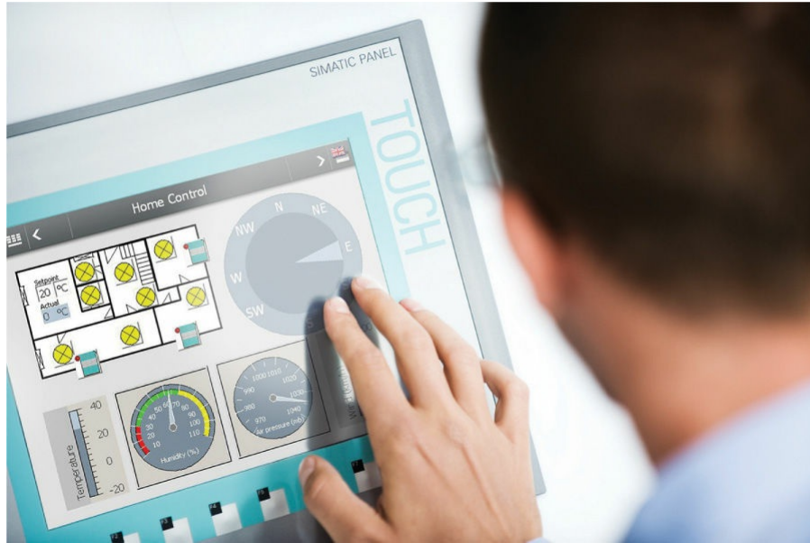
Figure 17-14 SIMATIC HMI Basic Panel with a touch screen (© Siemens AG 2014, All rights reserved)
