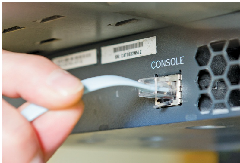
Figure 11-7 Plugging into a managed switch's console port using a serial cable
