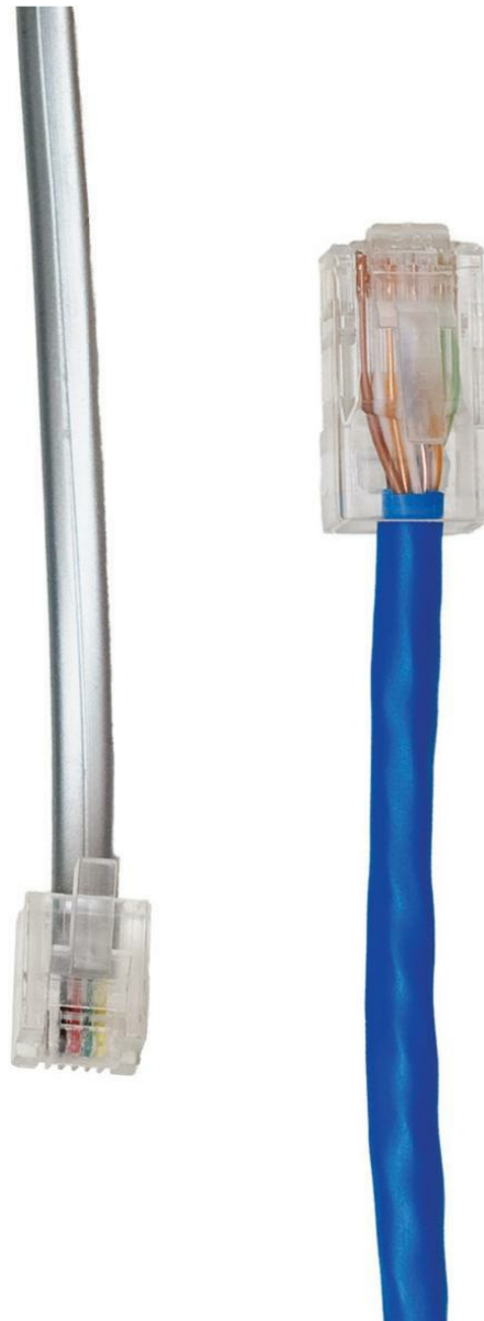
Figure 2-21 RJ-11 (left) and 8P8C/“RJ-45” (right) connectors
