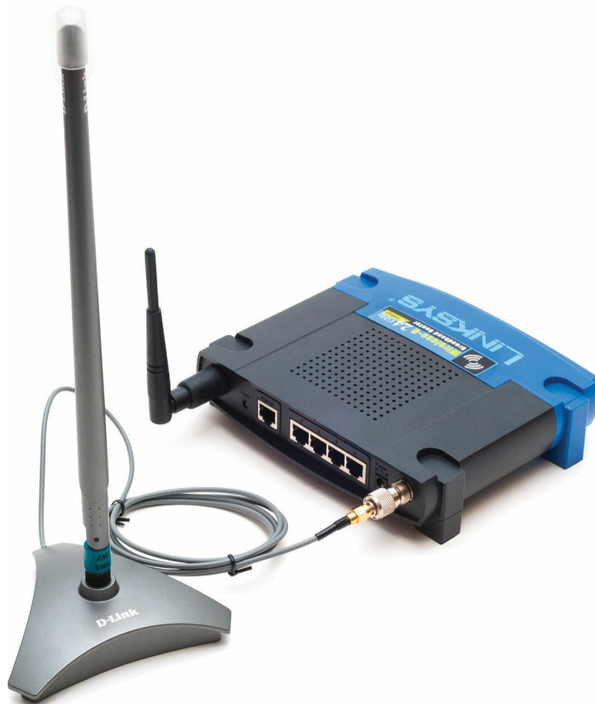
Figure 14-24 Replacement antenna on a WAP
