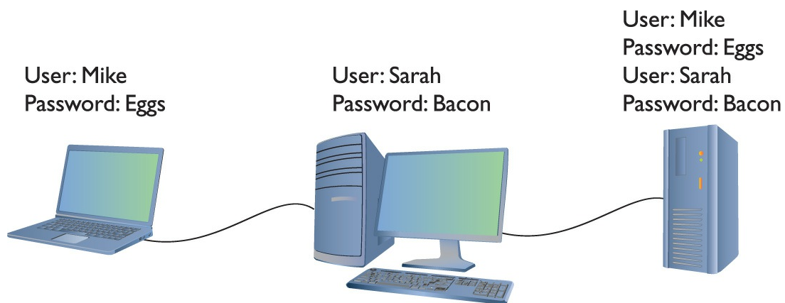
Figure 10-26 Users on an SSH server
