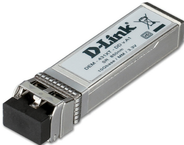
Figure 4-9 SFP+ transceiver (Photo courtesy of D-Link)
