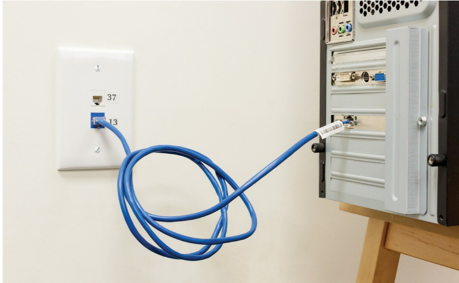
Figure 1-9 NIC with cable connecting the PC to the wall jack
