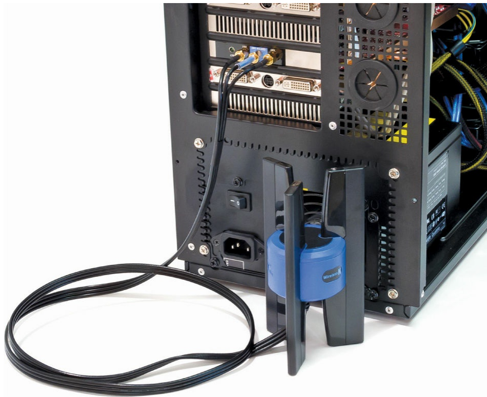
Figure 14-17 Wi-Fi NIC installed
