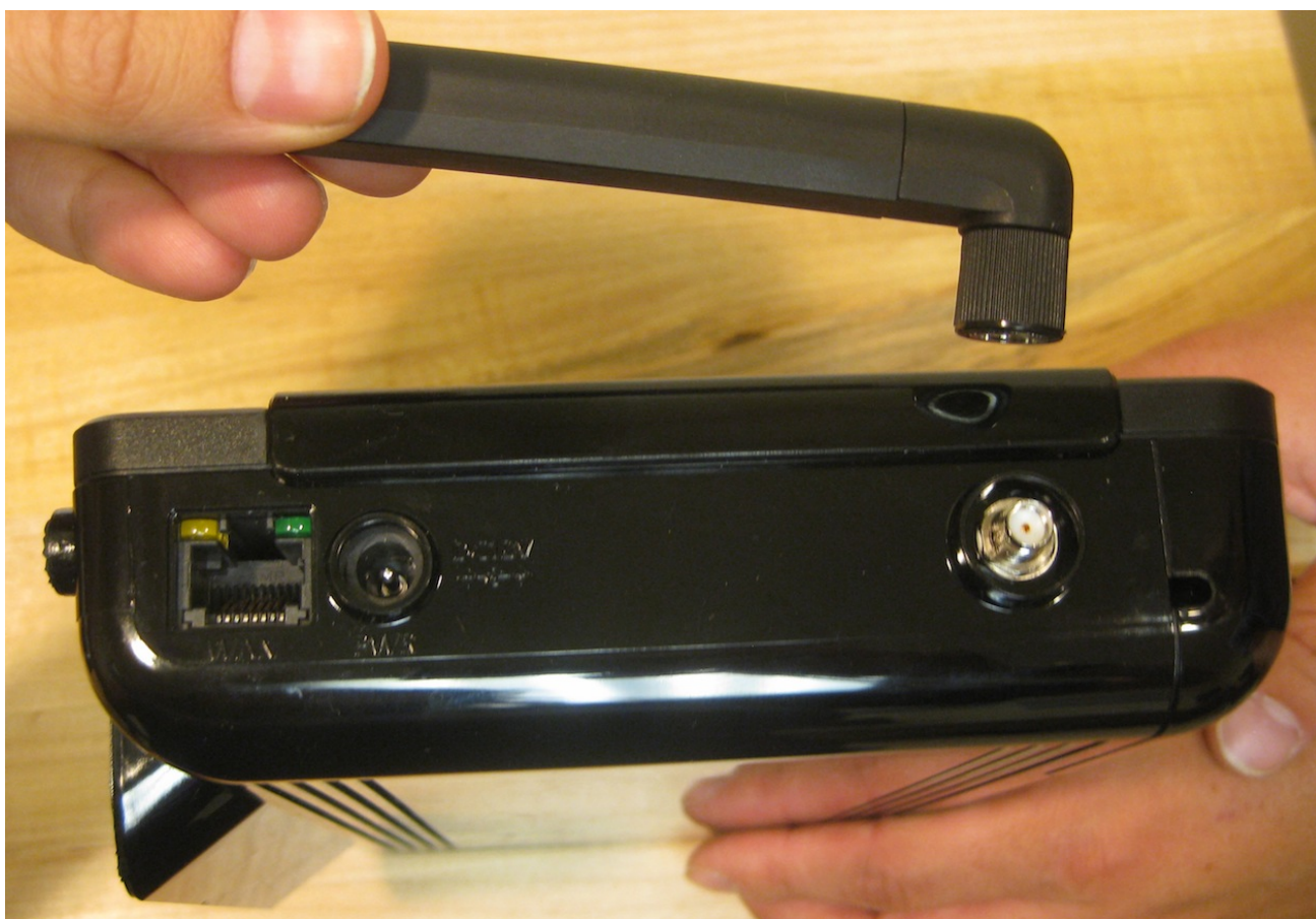
Figure 6: The Verizon Samsung SCS-26UC4 femtocell, showing Ethernet, power and RF antenna (from left to right).
