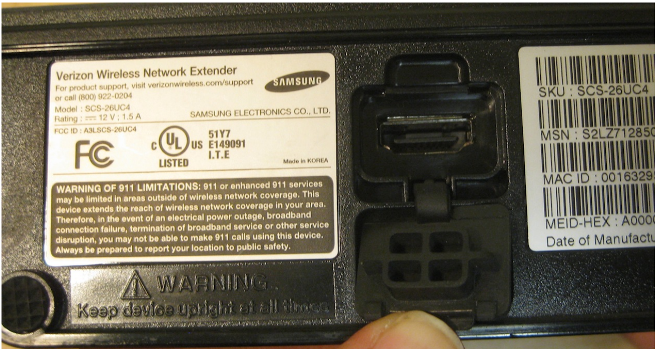
Figure 7: The base of the Verizon Samsung SCS-26UC4 femtocell, showing the HDMI port which LMG leveraged to gain console access.
