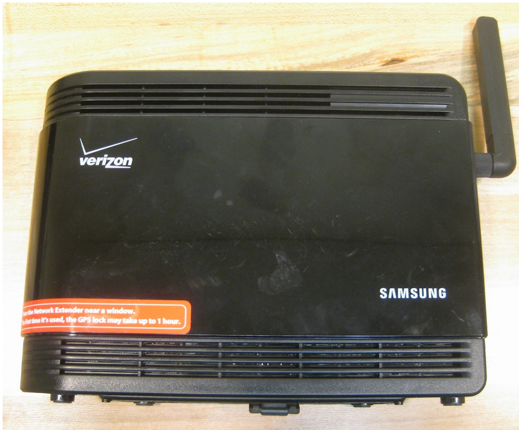
Figure 4: The Verizon Samsung SCS-26UC4 femtocell.
