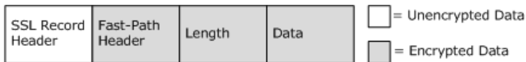
Figure 15: Encrypted fast-path packet
