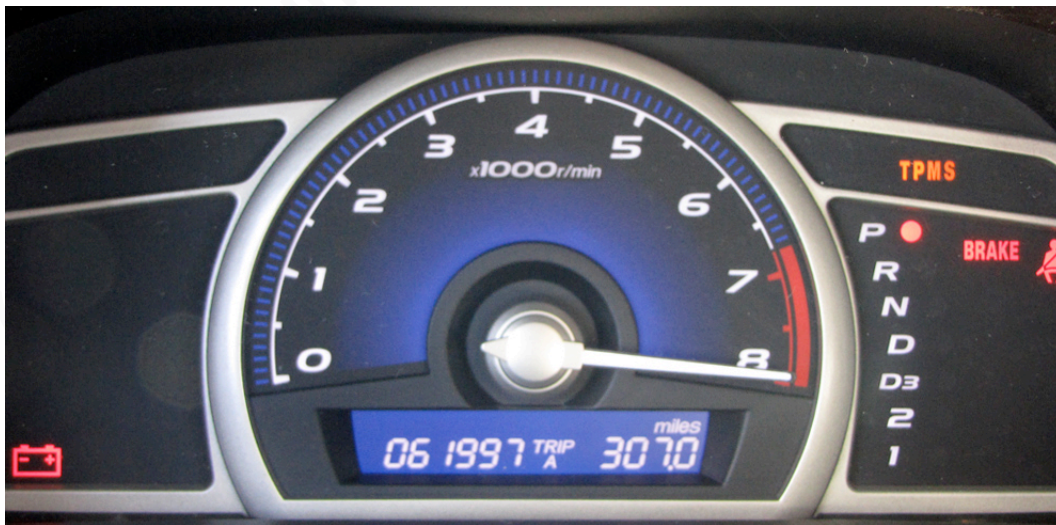
Figure 23: Successful Attack on Tachometer
