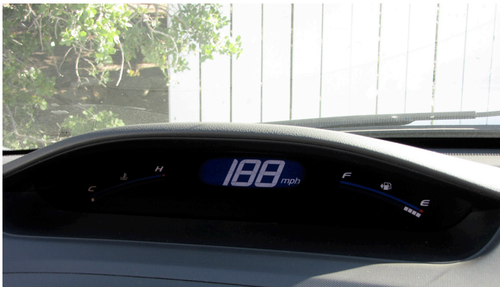
Figure 30: Successful Attack on Speedometer
